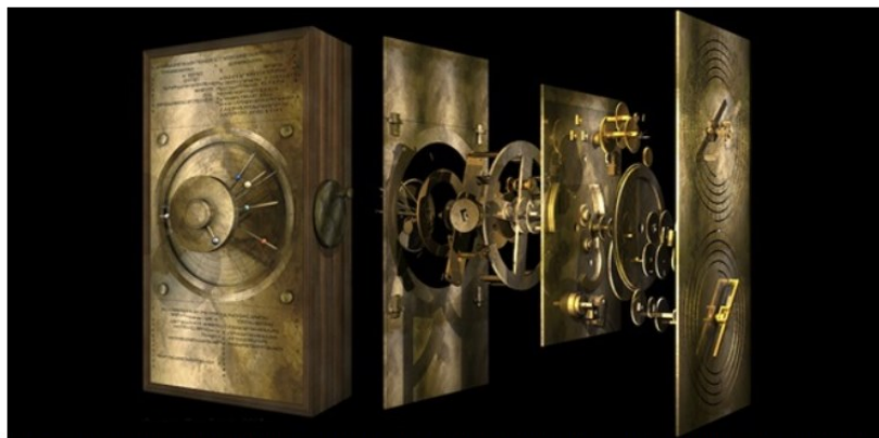
This exploded view shows what the Antikythera mechanism might have looked like. Here, the front plate (left) includes zodiac and calendar dials, as well as seven pointers. The back plate (right) has spiral scales for displaying solar and lunar eclipses and more. A new reconstructed view of the device featuring a revised front plate is expected to be published soon.
